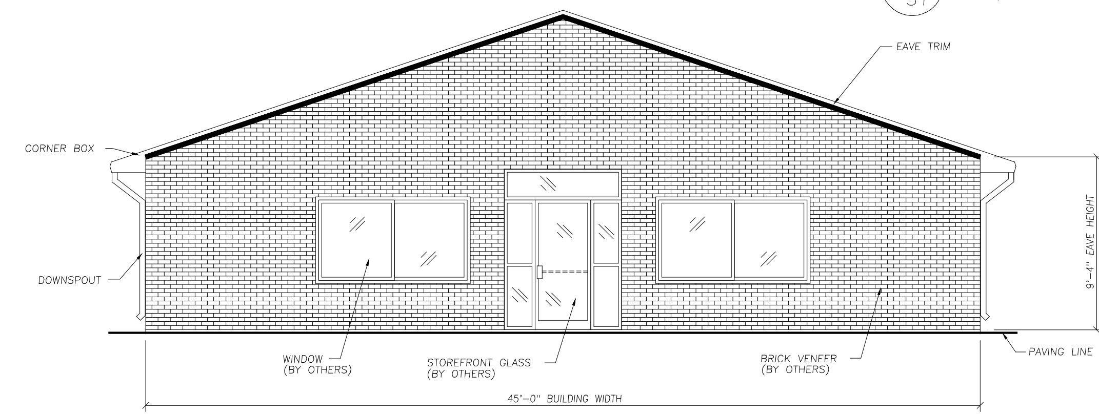
B ENDWALL ELEVATION . . . BUILDING "1" S1 SCALE: 1/4" = 1'-0"
